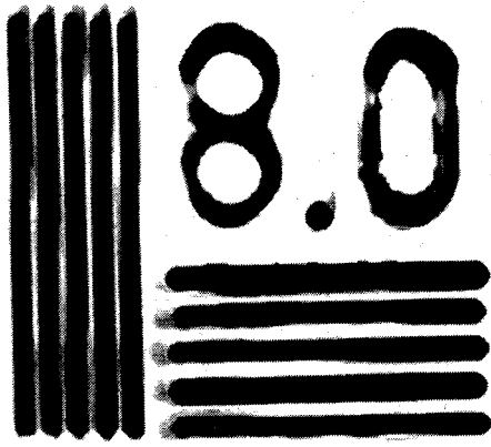
Fig. 2. A gray scale image of a section of the NIST 1963a test target (Cr coating on a glass substrate, linewidth is 63\ \mu\text{m} ). f = 79.6\ \text{GHz} ( \lambda = 3.8\ \text{mm} ), incident power is 0.5\ \text{mW} . The reference arm of the bridge is tuned to compensate reflection from the glass substrate. The spatial resolution is 128 \times 128 pixels.
